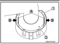
2. Hammer the portion (A) of exhaust finisher (1) to remove it in the rearward direction of vehicle.
